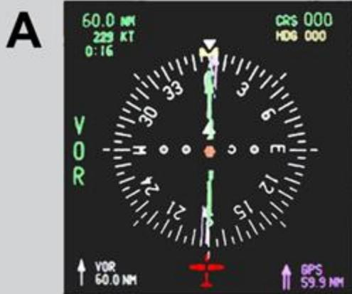
Tuned station at EHSI center. Aircraft on bearing pointer tail.
