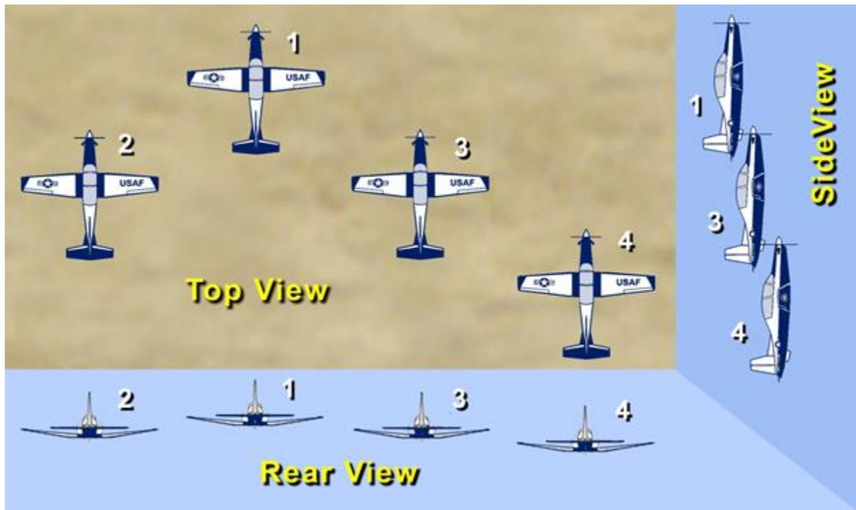
Figure A2.4. Four-ship Fingertip Formation in a Turn.
