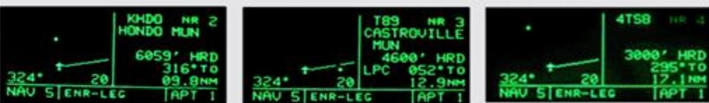
Pushing DIRECT then ENTER makes the displayed airfield the current waypoint. Allows for proceeding direct via a GPS course and to OBS the runway.
