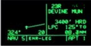
Pulling out and rotating the right inner knob cycles through nearest airfields:
