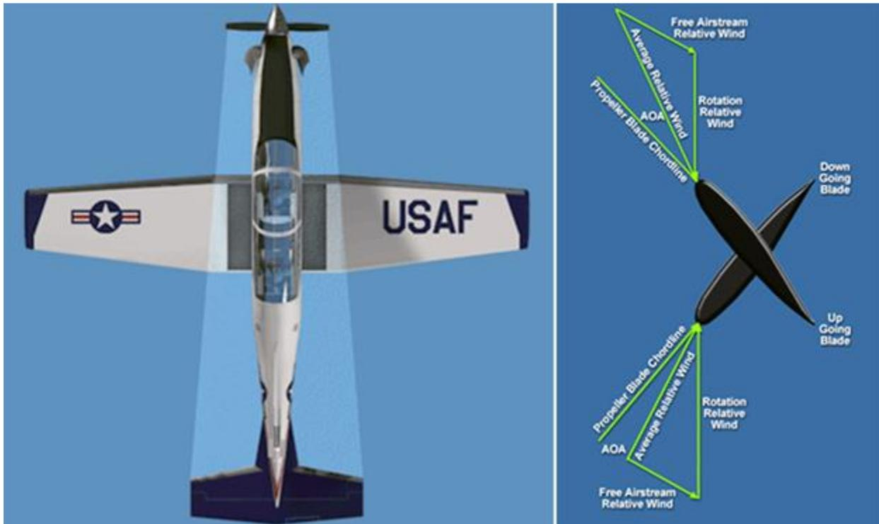
2.6.3. **Torque (Figure 2.5).** Torque reaction in a propeller-driven aircraft acts opposite the direction of propeller rotation. In the case of the T-6, the aircraft tends to roll to the left as a result of torque when power is increased, and the aircraft tends to roll right when power is reduced. Rudder and the TAD are the primary means for compensating for engine torque.
