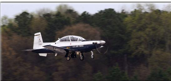
The T-6A Texan II is a single engine, two-seat primary trainer designed to train students in basic flying skills common to USAF pilots. Produced by Raytheon Aircraft, the T-6A Texan II is a military trainer version of Raytheon’s Beech/Pilatus Mk II. Columbus AFB received its first T-6 in October 2006 and now has 100 Texans in inventory.
