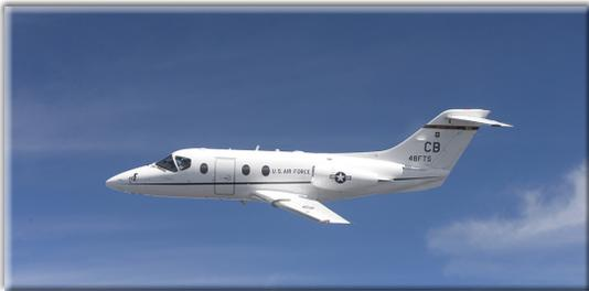
The T-1A Jayhawk is a medium range, twin-engine jet trainer used in the advanced phase of SUPT for students selected to fly airlift or tanker aircraft. The swept-wing T-1A is a military version of the Beech 400A. The T-1A differs from its commercial counterpart with structural enhancements that provide for a large number of landings per flight hour, increased bird strike resistance and an additional fuselage fuel tank. Columbus AFB has 47 Jayhawks.
