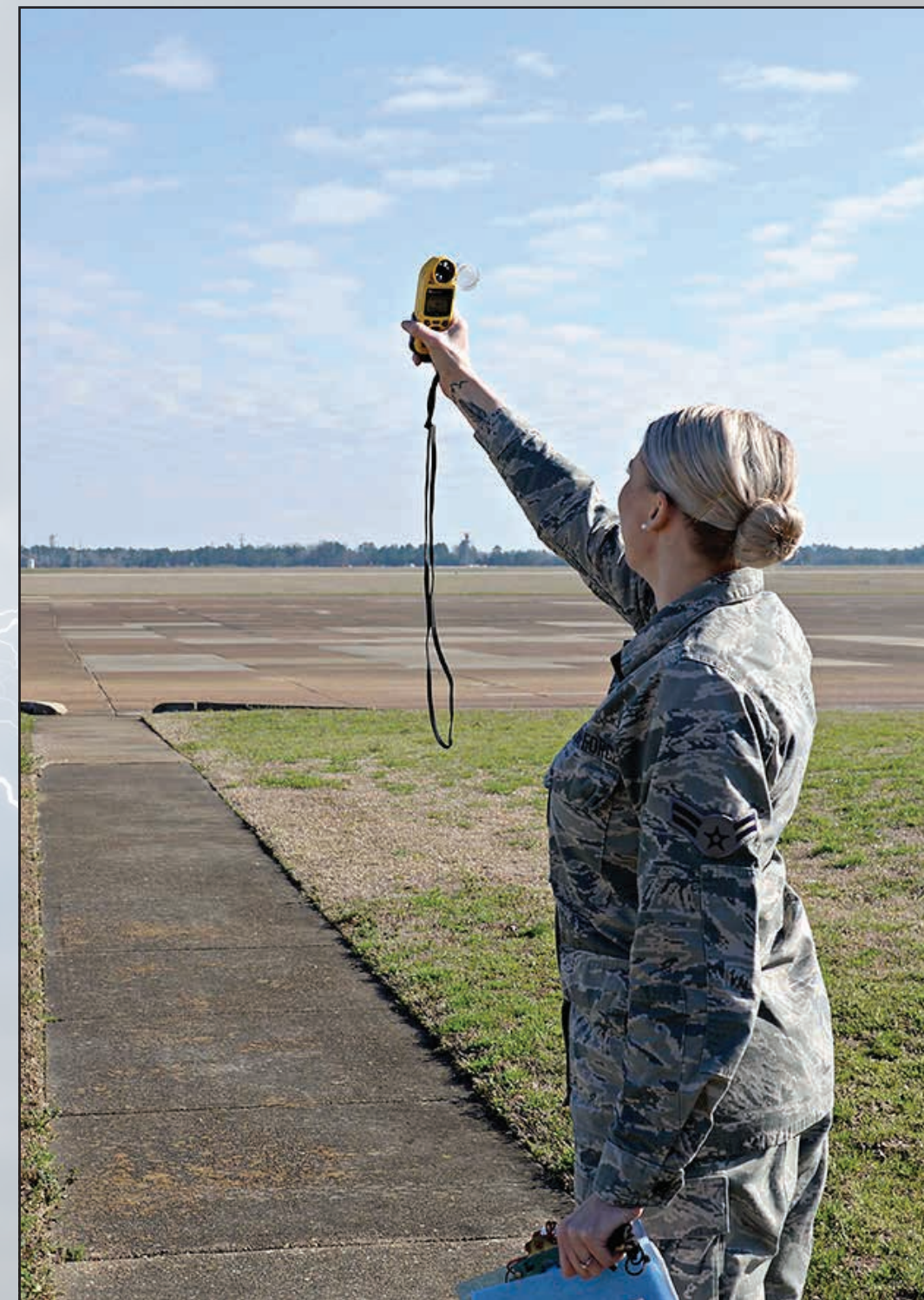
Airman 1st Class Lauren Rodgers, 14th Operations Support Squadron Weather Flight apprentice, gauges the wind with an anemometer Feb. 27, 2019, on Columbus Air Force Base, Mississippi. Anemometer are used to measure wind speed.
