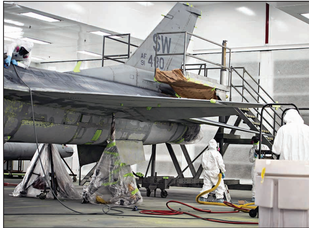
U.S. Air Force photo by Senior Airman Christopher Maldonado Airmen assigned to the 20th Equipment Maintenance Squadron corrosion control paint barn, work on an F-16CM Fighting Falcon at Shaw Air Force Base, South Carolina, Nov. 13, 2018. The maintenance performed on the aircraft helps protect the aircraft from the elements while stateside or overseas.
