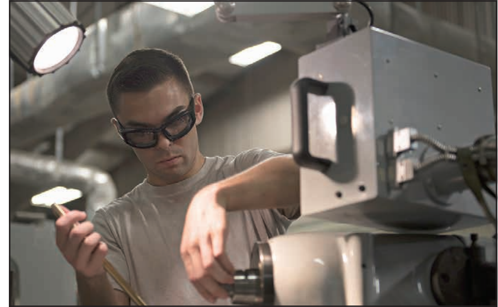
U.S. Air Force Senior Airman Timothy Bergin, 33rd Maintenance Squadron aircraft metals technologist, attaches a metal rod to a machine Oct. 3, 2018, at Eglin Air Force Base, Fla. The metal rod is used to make pins that insert into the actuating levers for stability.
