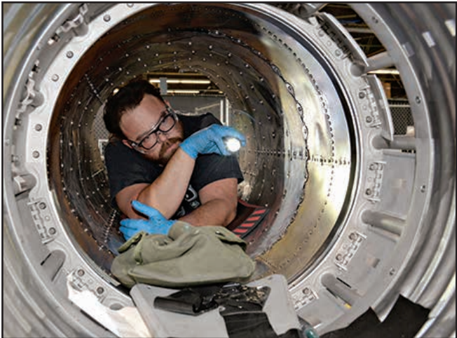
Jason Moore, 575th Aircraft Maintenance Squadron maintenance support flight, inspects the inside of T-38 Talon boat tail section April 17, 2018, at Joint Base San Antonio-Randolph, Texas.
