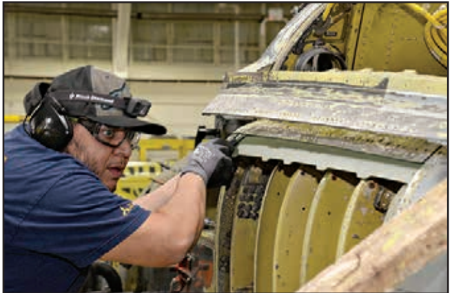
Michael Ramirez, 575th Aircraft Maintenance Squadron sheet metal technician, checks the alignment on a new left hand upper center longeron being installed on a T-38 Talon during the Pacer Classic III modification package April 17, 2018, at Joint Base San Antonio-Randolph, Texas.
