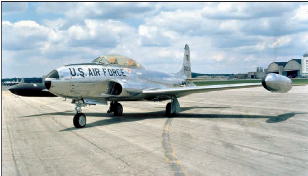
U.S. Air Force photo A T-33A Shooting Star sits at the National Museum of the United States Air Force in Dayton, Ohio. The two-place T-33 Shooting Star jet was designed for training pilots already qualified to fly propeller-driven aircraft.
