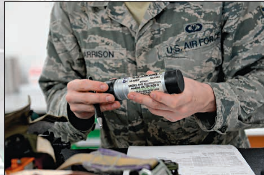
BELOW: Senior Airman Hayden Harrison, 48th Flying Training Wing Aircrew Flight Equipment technician, checks a part from a T-6A Texan II survival equipment checklist Dec. 5, 2017, on Columbus Air Force Base, Mississippi. Every piece of a survival kit has a matching serial number and expiration date that must be checked and updated as necessary.
