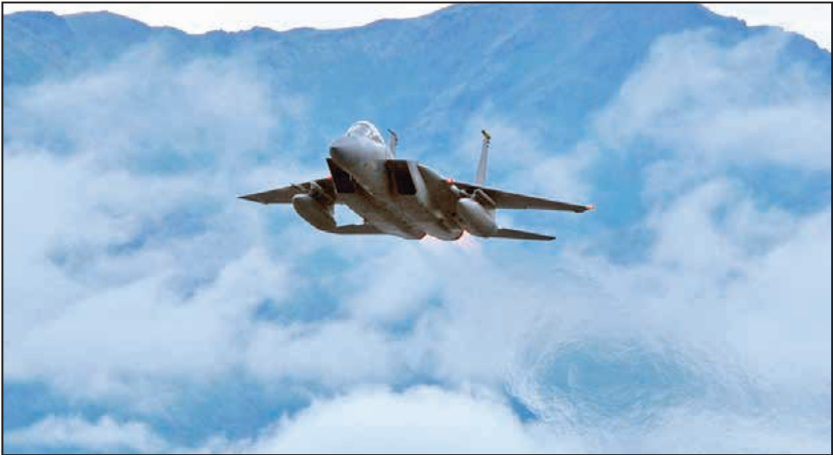
U.S. Air Force photo by Senior Airman Laura Turner An F-15 Eagle aircraft takes off from Elmendorf Air Force Base, Alaska. The F-15’s superior maneuverability and acceleration are achieved through high engine thrust-to-weight ratio and low wing loading.
