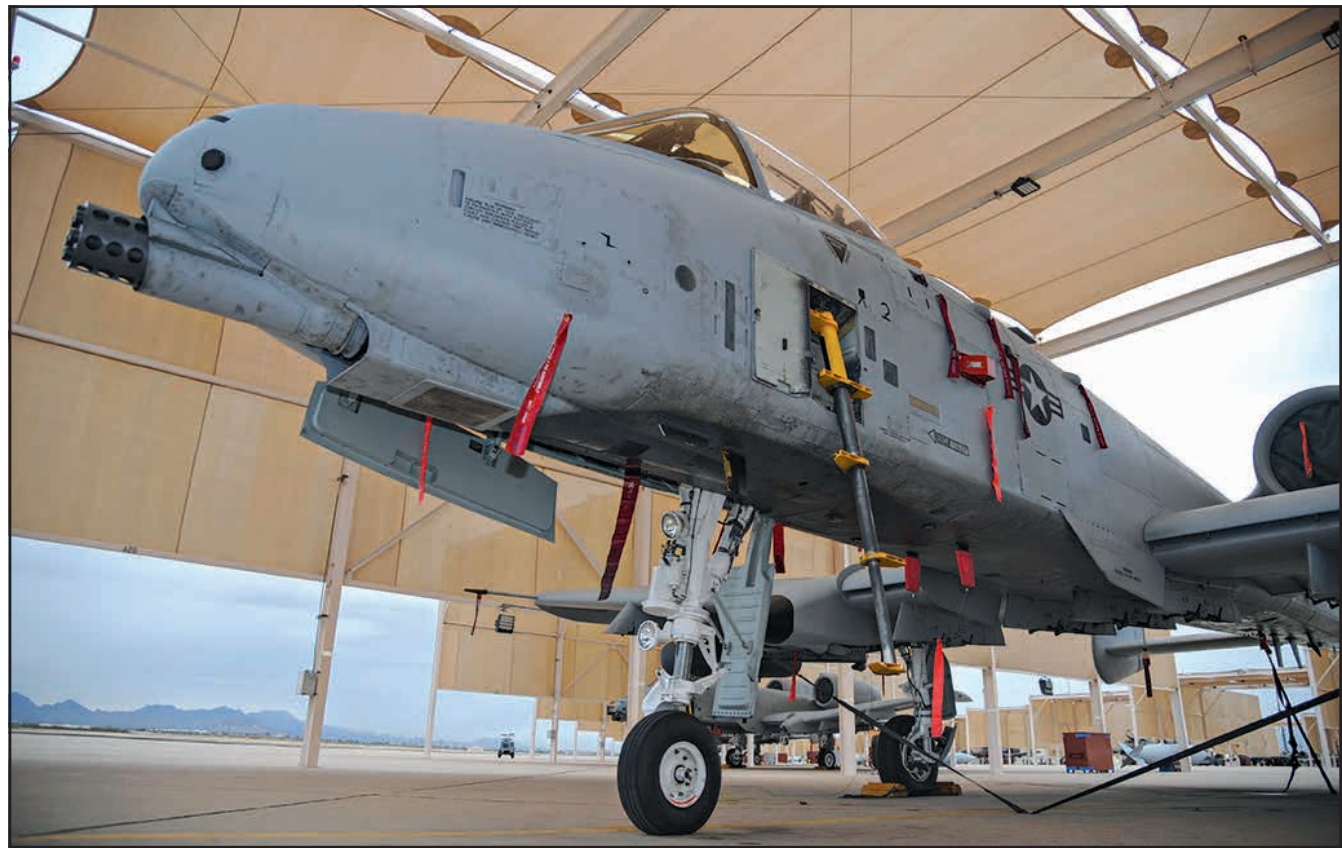
U.S. Air Force photo by Airman 1st Class Mya M. Crosby An A-10C Thunderbolt II, upgraded with a new lightweight airborne recovery system V-12, rests on the flight line at Davis-Monthan Air Force Base, Arizona, Dec. 21, 2016. The LARS V-12 is designed to allow A-10 pilots a more effective means of communication with individuals on the ground such as downed pilots, pararescuemen and joint terminal attack controllers.
