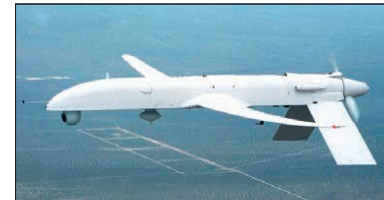
Courtesy Photo The GNAT 750 was the first long-endurance remotely piloted aircraft. After it was purchased by the Air Force, it would evolve into the RQ-1 Predator during the 1990s to fly its first missions over the Balkans during the Kosovo conflict.
