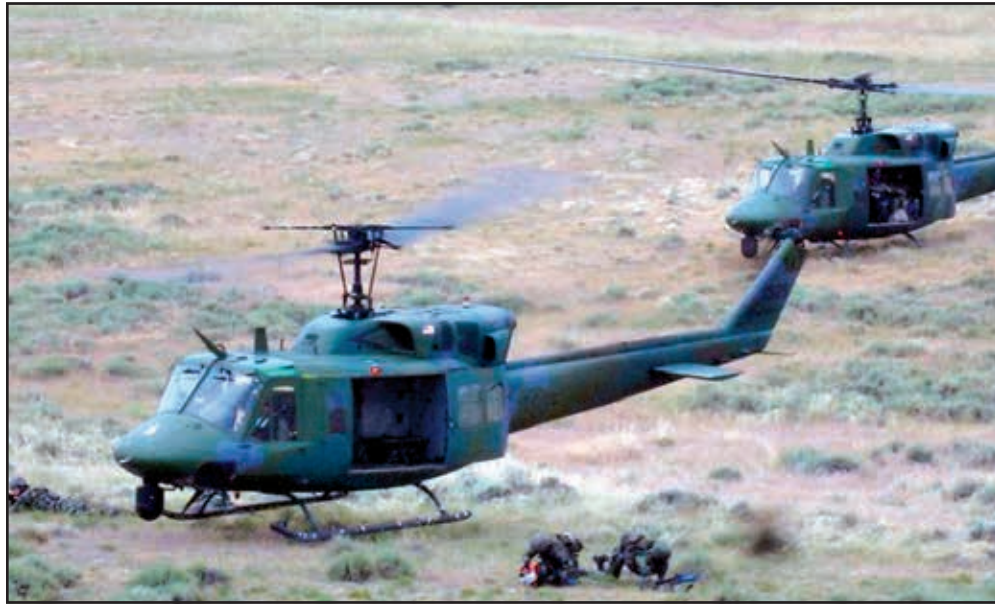
The UH-1N Twin Huey helicopter is a light-lift utility helicopter used to support various missions. The primary missions include airlift of emergency security forces, security and surveillance of off-base nuclear weapons convoys, and distinguished visitor airlift.
