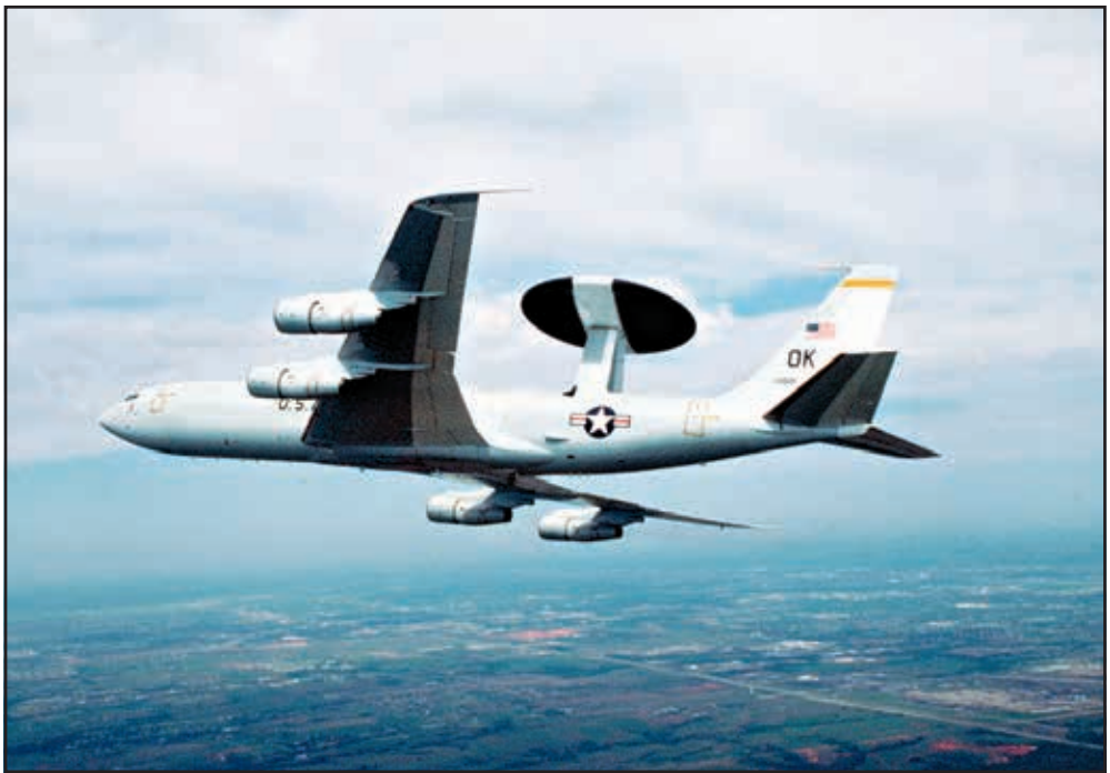
U.S. Air Force photo/Tech. Sgt. John McDowell An E-3 Airborne Warning and Control System aircraft from Tinker Air Force Base, Oklahoma, flies a mission. The E-3 Sentry is a modified Boeing 707/320 commercial airframe with a rotating radar dome.
