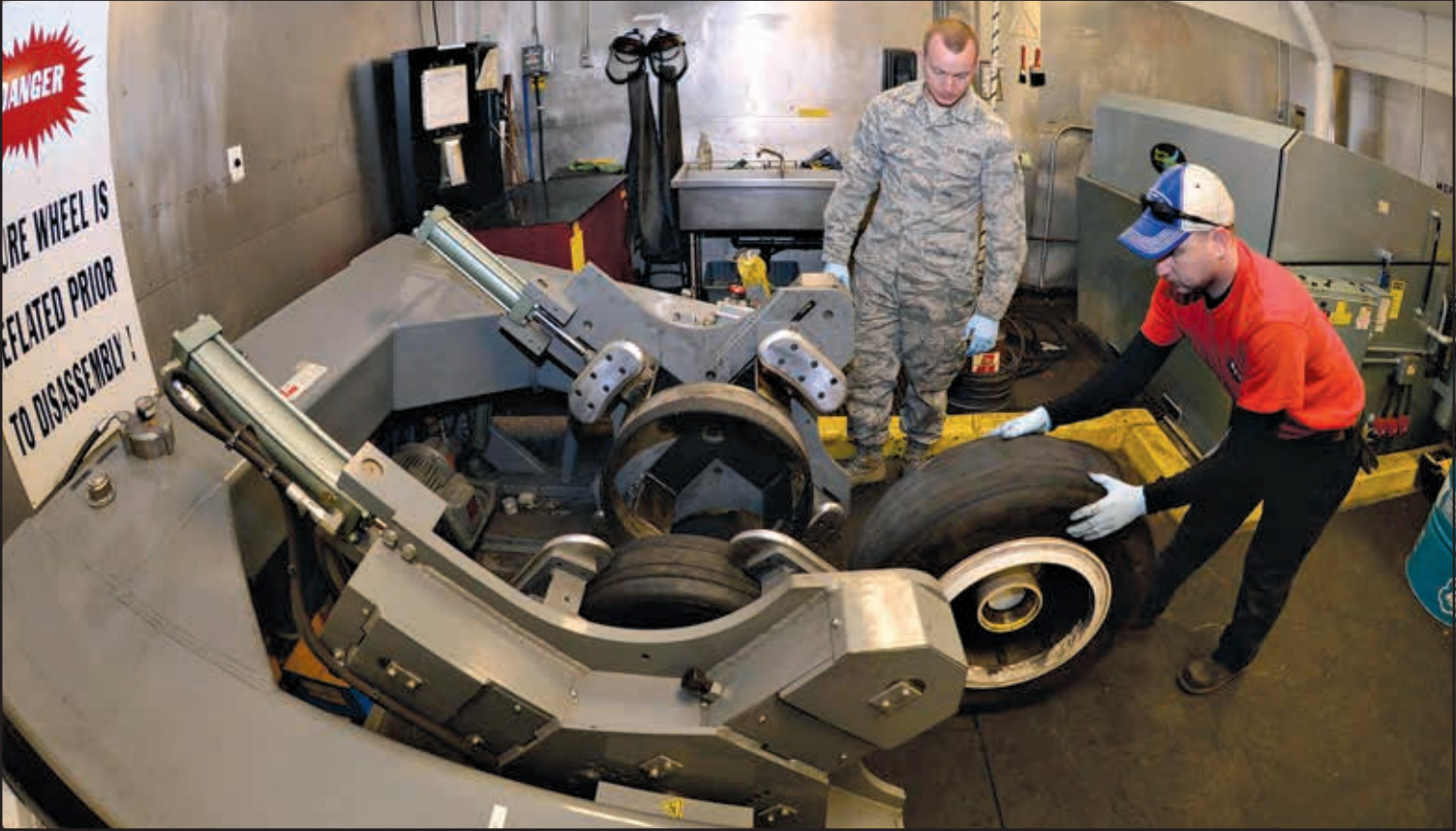
U.S. Air Force photo/Todd Cromar Tech. Sgt. James Speicher, right, an air reserve technician with the 419th Maintenance Squadron, rolls an F-35 Lightning II wheel into a tire changing machine May 20, 2016, while Senior Airman Joseph Sprowls, of the 388th Maintenance Squadron, looks on in the wheel and tire shop at Hill Air Force Base, Utah. The machine depicted is a legacy tool which has been adapted via a fabricated bead breaker to be used in changing F-35 tires.
