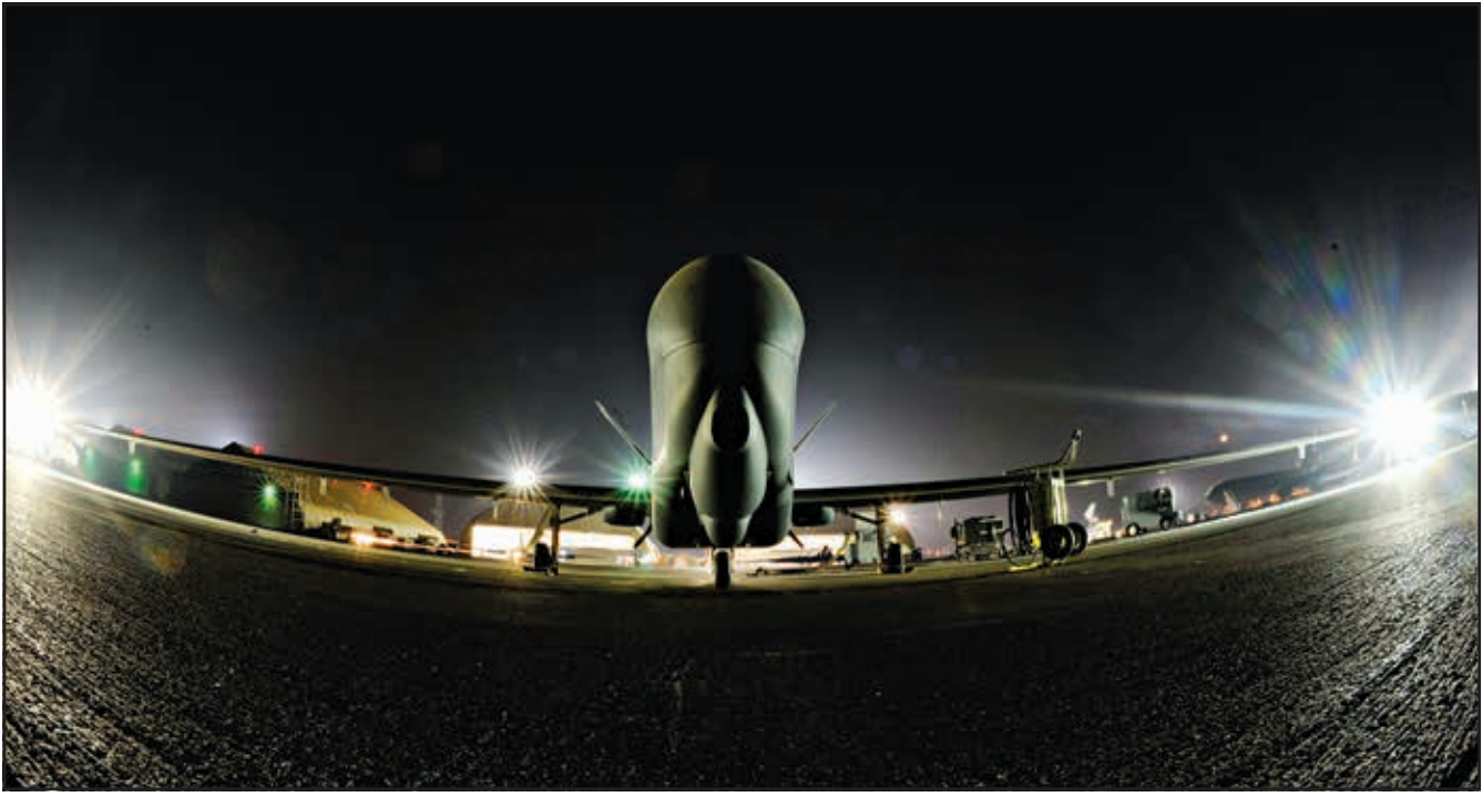
U.S. Air Force photo A U.S. Air Force RQ-4 Global Hawk Unmanned Aerial Vehicle waits for its takeoff time before its first launch from an undisclosed location in Southwest Asia, Nov. 27, 2010. The RQ-4 carries the Battlefield Airborne Communications Node which acts as a persistent gateway, bridging diverse tactical data links and voice communications to improve battlefield communications.
