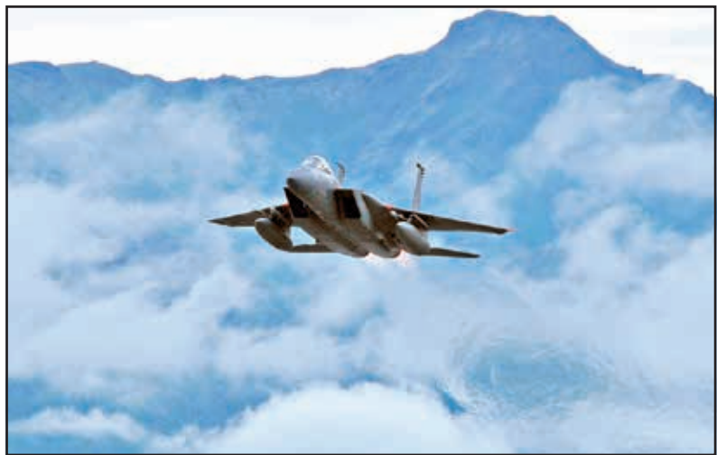
An F-15 Eagle takes off from Elmendorf Air Force Base, Alaska. The F-15's superior maneuverability and acceleration are achieved through high engine thrust-to-weight ratio and low wing loading.
