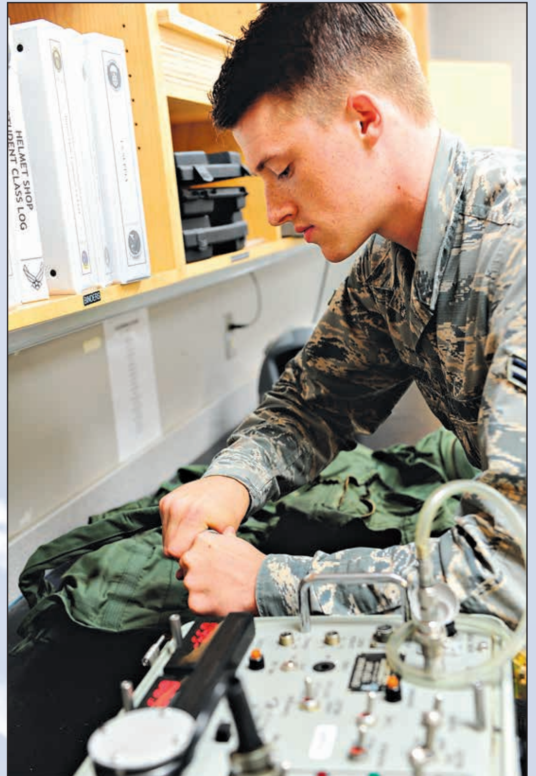
U.S. Air Force photo/Airman 1st Class John Day Airman 1st Class Hayden Harrison, 14th Operations Support Squadron Aircrew Flight Equipment Technician, tests a g-suit for the proper pressure June 4 at Columbus Air Force Base, Mississippi. AFE fits, inspects, maintains and repairs all of the flight gear that connects the pilot to the aircraft.
