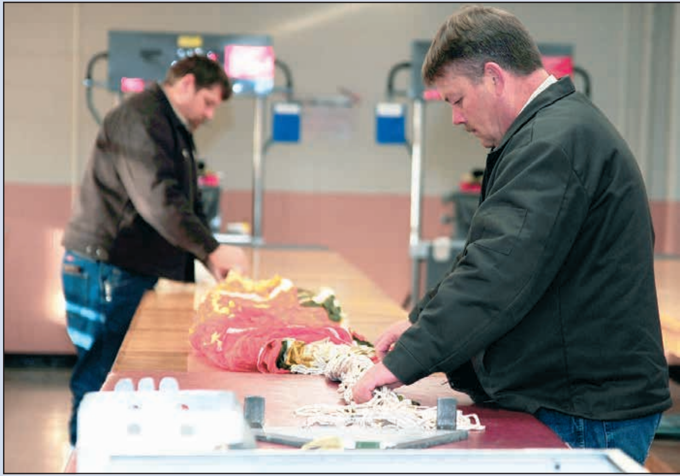
U.S. Air Force photo/Senior Airman Stephanie Englar Roger Collier and Lee Horn, both contractors working for the 14th Operations Support Squadron, inspect a parachute canopy before packing it into a parachute head-box on Columbus Air Force Base, Mississippi. The entire process for packing a parachute spans over the course of two days and requires a three-ton press.
