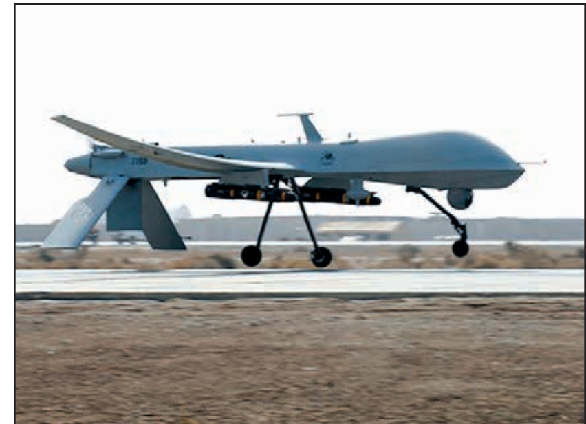
U.S. Air Force photo/Airman 1st Class Jonathan Snyder An Air Force MQ-1B Predator from the 361st Expeditionary Reconnaissance Squadron takes off from Ali Base, Iraq, in support of Operation Iraqi Freedom. The Predator is a medium-altitude, long-endurance, remotely piloted aircraft capable of conducting armed reconnaissance.
