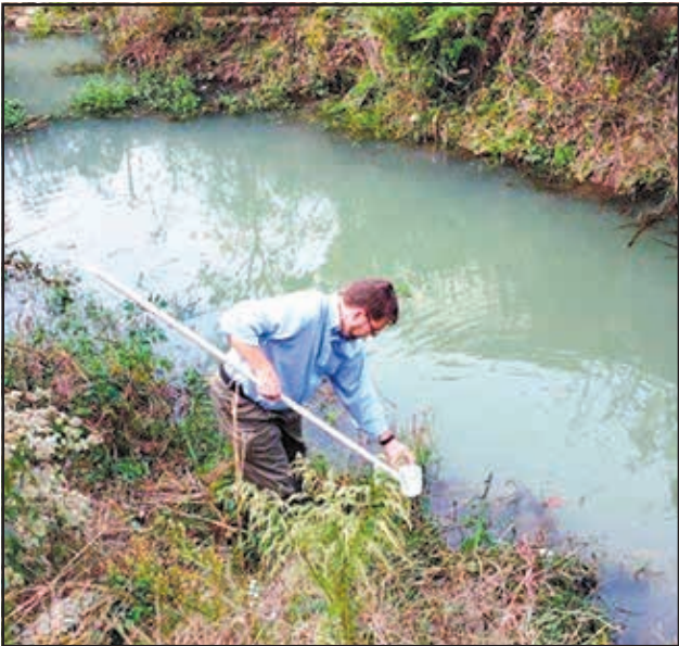
Courtesy photo Mike Jago, 14th Civil Engineer Squadron Environmental Element Chief, takes a water sample from one of the outfalls on Columbus Air Force Base, Mississippi. By using a pitcher attached to the end of a long pole, samples can be collected from the outfalls without exposure to potentially hazardous waters.
