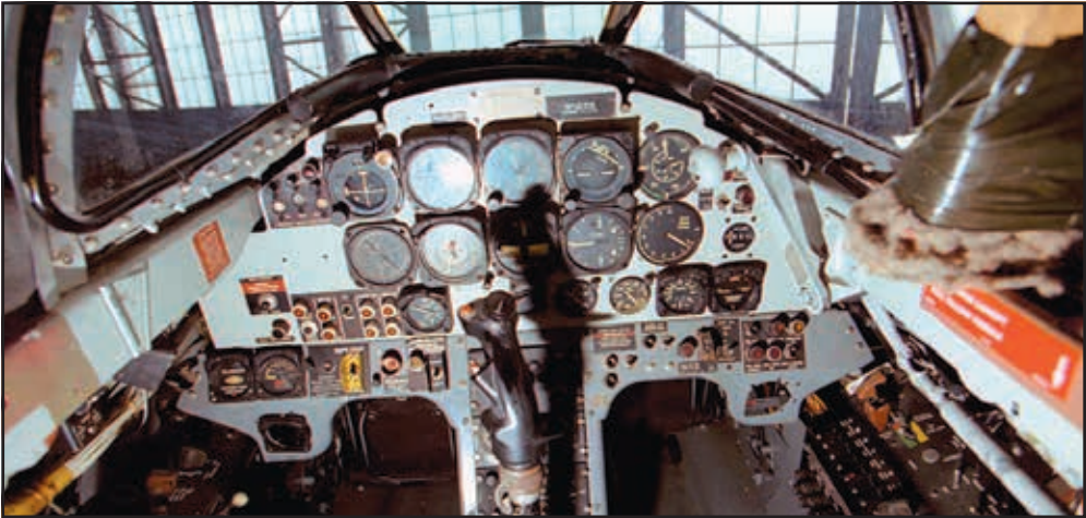
U.S. Air Force photo DAYTON, Ohio – A Lockheed T-33A Shooting Star front cockpit sits at the National Museum of the United States Air Force in Dayton, Ohio. It was developed from the single-seat F-80 fighter by lengthening the fuselage about three feet to accommodate a second cockpit.
