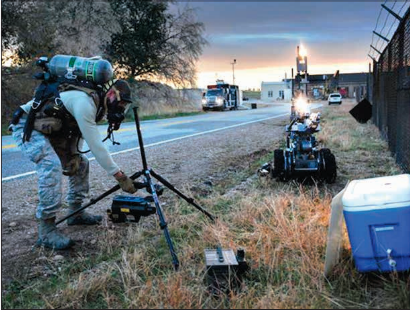
U.S. Air Force photo/Micah Garbarino With the aid of lights and cameras on a remote-controlled robot, Senior Airman Garret Corbett, an explosive ordnance disposal technician with the 775th EOD Flight at Hill Air Force Base, sets up a mobile to examine the contents of a cooler during a training scenario on investigating suspicious packages. Once Corbett takes the X-ray, he can process them in a mobile computer lab in the command truck.
