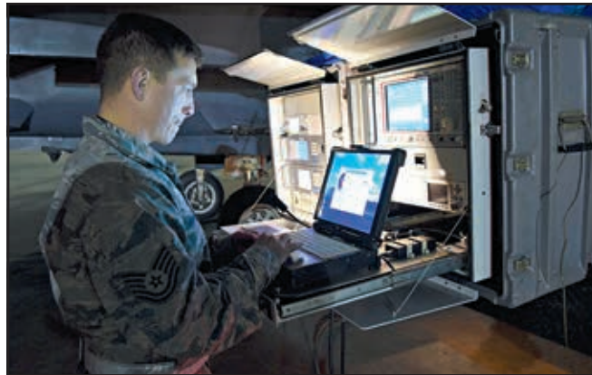
U.S. Air Force photo/Senior Airman Aaron J. Jenne Tech. Sgt. Matthew Hoover, a Combat Shield crew leader assigned to the 16th Electronic Warfare Squadron, Eglin Air Force Base, Florida, monitors a USM-642 Raven signal generator during Combat Shield, Oct. 20, 2015, at Seymour Johnson Air Force Base, North Carolina. Hoover used the USM-642 to simulate real-world radar emissions and test the sensitivity of the threat detection systems of an F-15E Strike Eagle.
