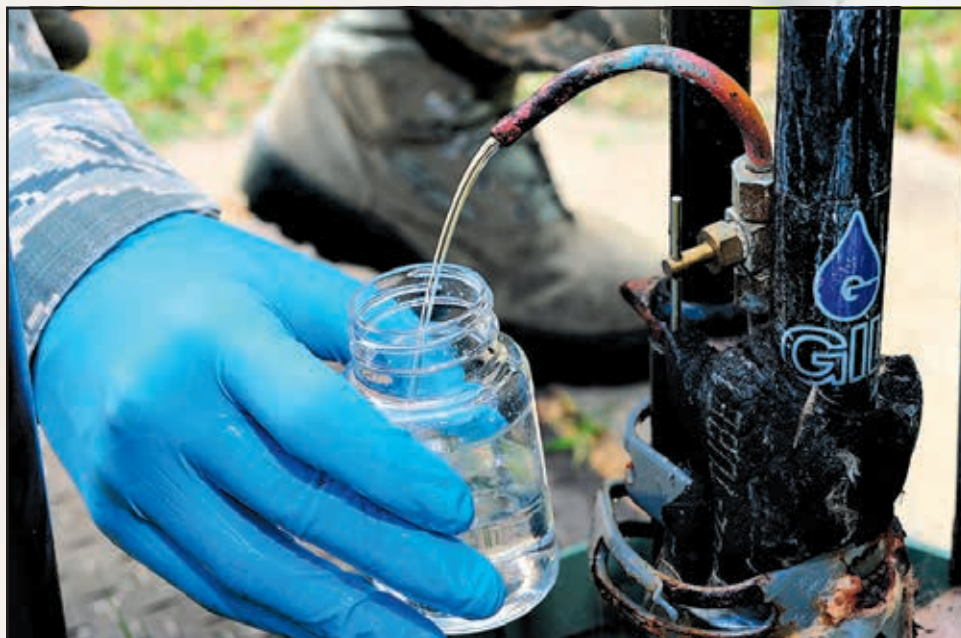
Airman 1st Class Rolando Chavez, 14th Medical Operations Squadron Bioenvironmental Technician, gathers water Aug. 5 at Columbus Air Force Base, Mississippi, to be sent to the Mississippi State Department of Health. Bioenvironmental checks the water supply on base bimonthly to ensure proper contaminate control.
