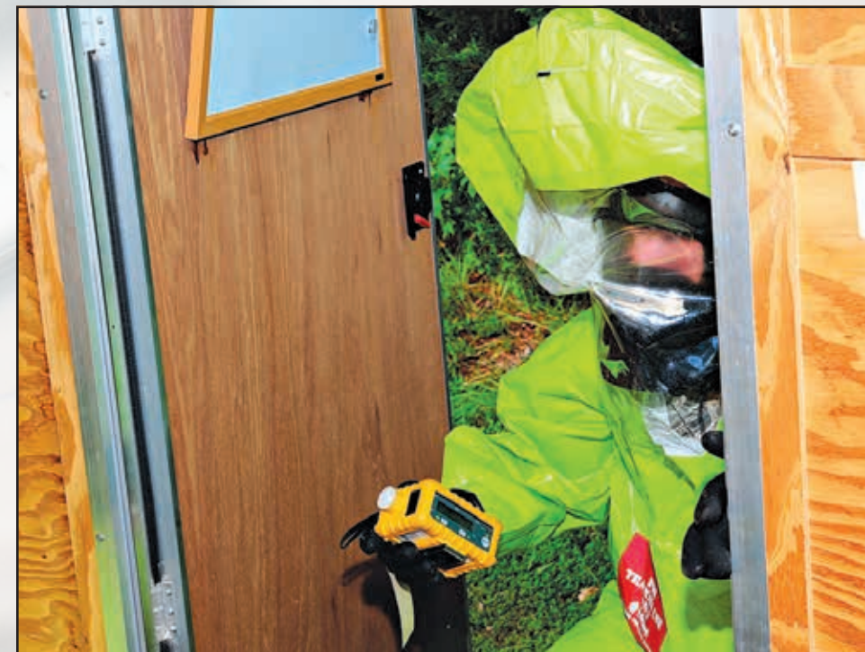
Senior Airman Kevin Morgan, 14th Medical Operations Squadron Bioenvironmental Technician, checks a confined area with a multi-gas reader in a Level-A response suit Aug. 5 at Columbus Air Force Base, Mississippi. Gas detectors can be used by Airmen to detect combustible, flammable and toxic gases in the area.
