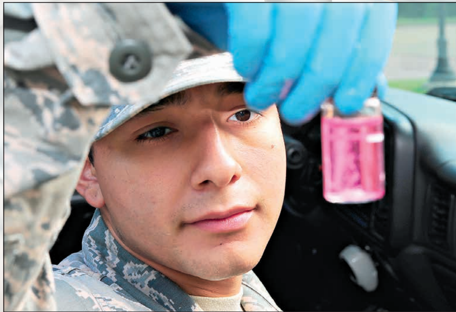
Airman 1st Class Rolando Chavez, 14th Medical Operations Squadron Bioenvironmental Technician, tests the chlorine level of the base's water supply outside of State Village Aug. 5 at Columbus Air Force Base, Mississippi. Too much chlorine can affect the taste of the water and cause drinkers to seek other sources of water, but not enough chlorine will allow bacteria and other microorganisms to survive causing water supplies to carry diseases.
