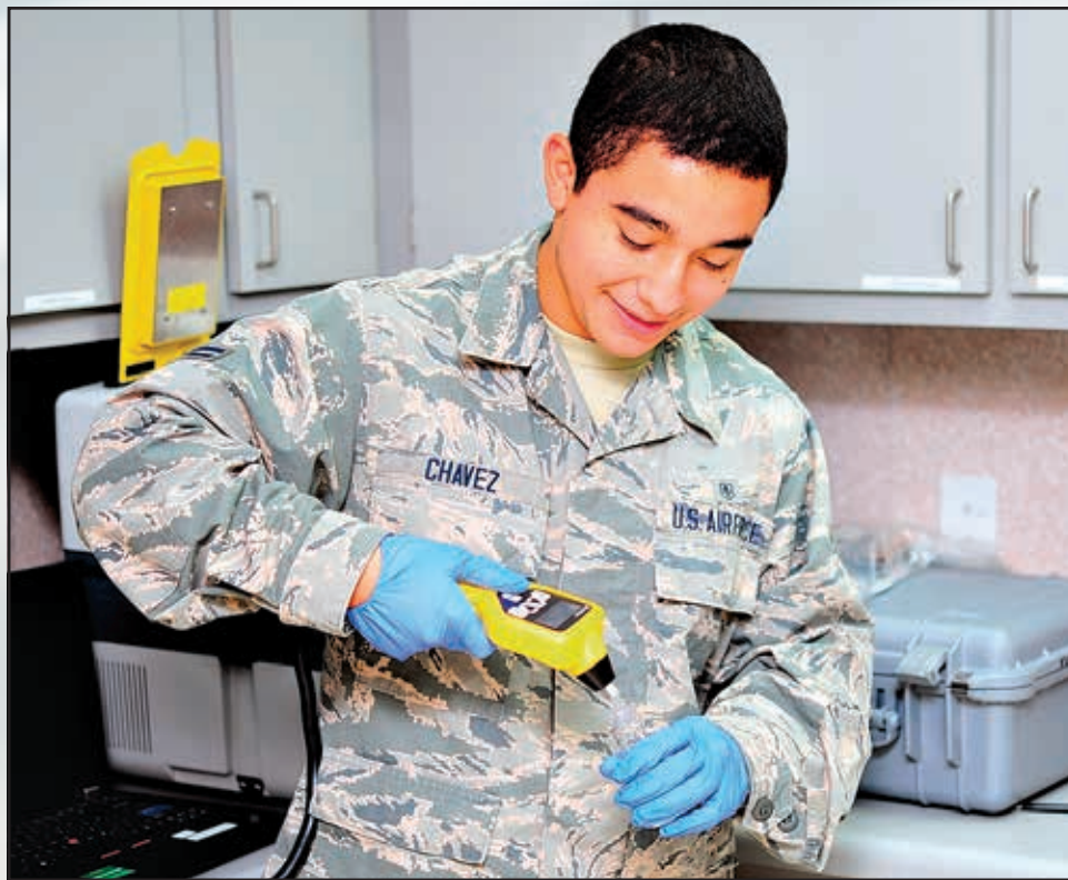
Airman 1st Class Rolando Chavez, 14th Medical Operations Squadron Bioenvironmental Technician, uses a chemical identification system to check for contaminate vapors Aug. 5 at Columbus Air Force Base, Mississippi. The instrument makes it faster for users to detect and identify toxic industrial chemicals and chemical warfare agents right at the scene of an incident.
