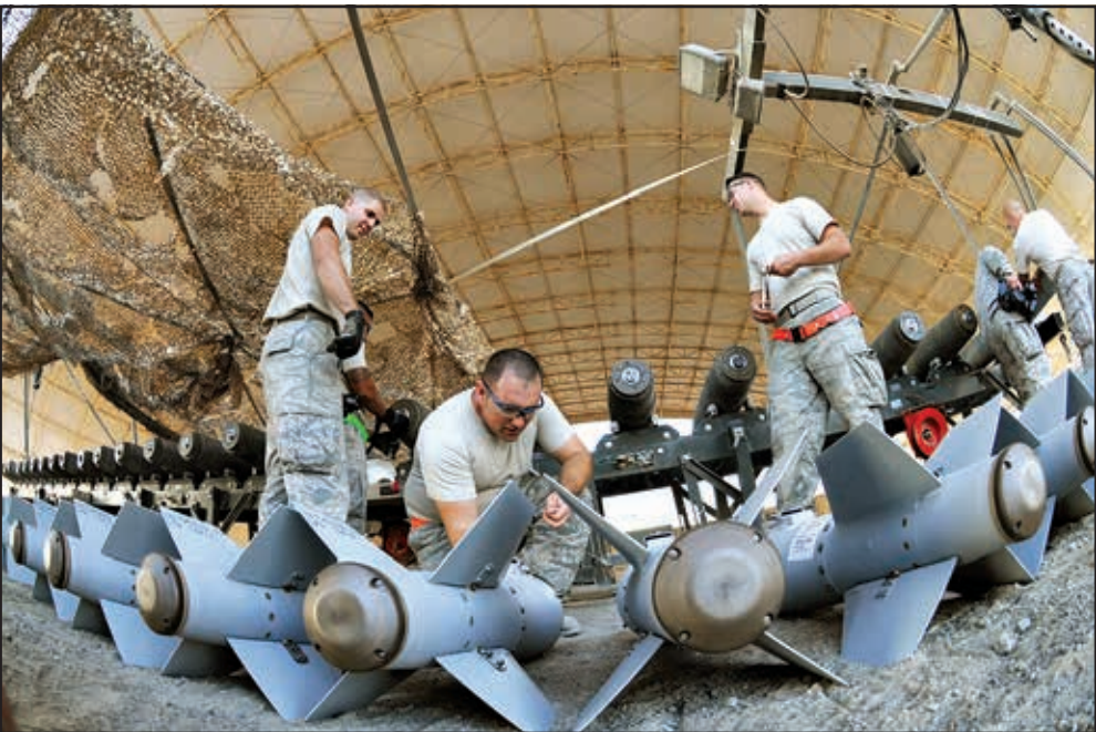
Master Sgt. Adam, middle, preps the KMU-572 fins for assembly onto the MK-82 munition Dec. 21, 2014, in Southwest Asia. Adam is the NCO in charge of conventional maintenance and is deployed from Seymour Johnson Air Force Base, N.C.
