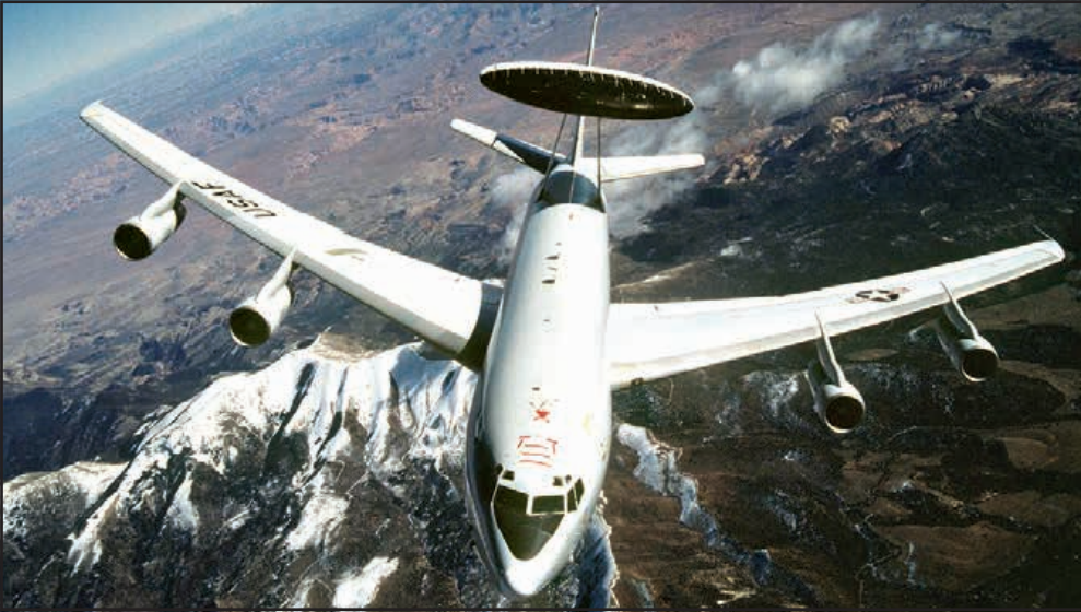
Courtesy photo The E-3 Sentry is a modified Boeing 707/320 commercial airframe with a rotating radar dome. The dome is 30 feet in diameter, 6 feet thick and is held 11 feet above the fuselage by two struts. It contains a radar subsystem that permits surveillance from the Earth's surface up into the stratosphere, over land or water. The radar has a range of more than 200 miles for low-flying targets and farther for aerospace vehicles flying at medium to high altitudes.
