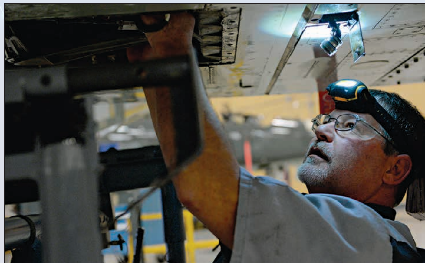
Steve Henderson, L3 Technologies T-38C Talon maintainer, finishes switching the stability augmentation system on a T-38 Feb. 14, 2018, on Columbus Air Force Base, Mississippi. Maintainers must take the outside hull of the aircraft apart, similar to a shell, to reach pieces such as the engine to complete some of their maintenance.
