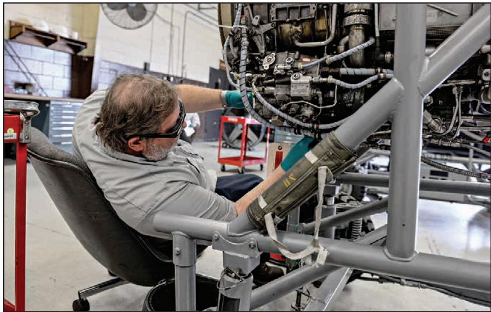
U.S. Air Force photo by Airman 1st Class Davis Donaldson Frank Hall, M1 Support Services propulsion mechanic, performs maintenance on a General Electric J85-GE-5 turbojet engine April 17, 2020, at Columbus Air Force Base, Miss. Propulsion means to push or drive an object forward, and these engines help power the wing's T-38 Talons.
