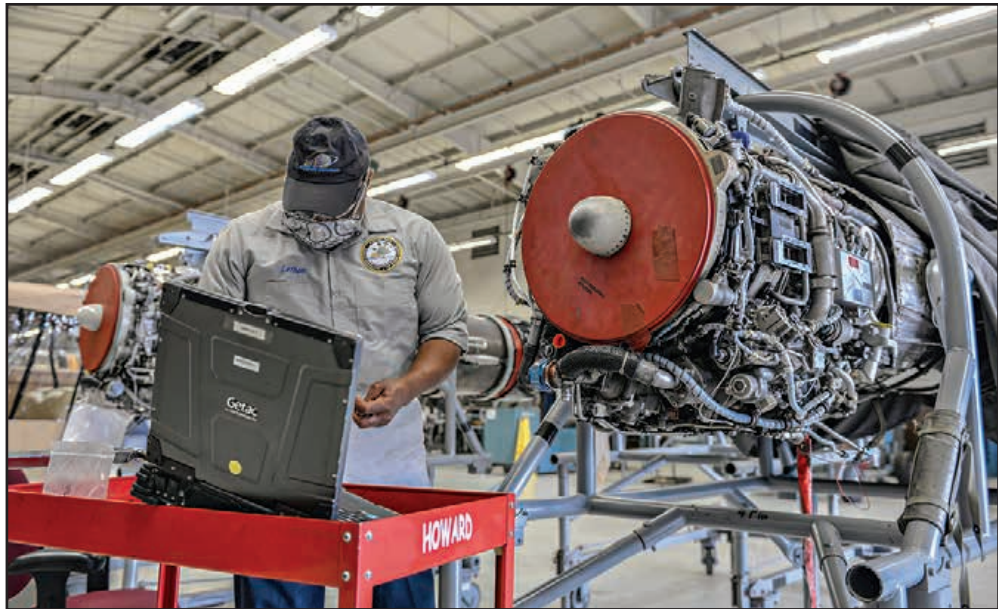
U.S. Air Force photo by Airman 1st Class Davis Donaldson Willy Latham, M1 Support Services propulsion mechanic, gathers tools in order to perform maintenance on a General Electric J85-GE-5 turbojet engine April 17, 2020, at Columbus Air Force Base, Miss. The T-38 Talon is equipped with two General Electric J85-GE-5 turbojet engines.
