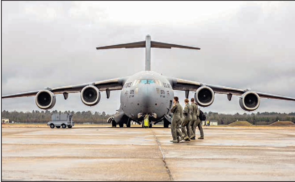
U.S. Air Force photo by Airman Davis Donaldson Four Airmen walk in front of a C-17 Globemaster III Dec. 10, 2019, at Columbus Air Force Base, Miss. The C-17 measures 174 feet long (53 meters) with a wingspan of 169 feet, 10 inches (51.75 meters).
