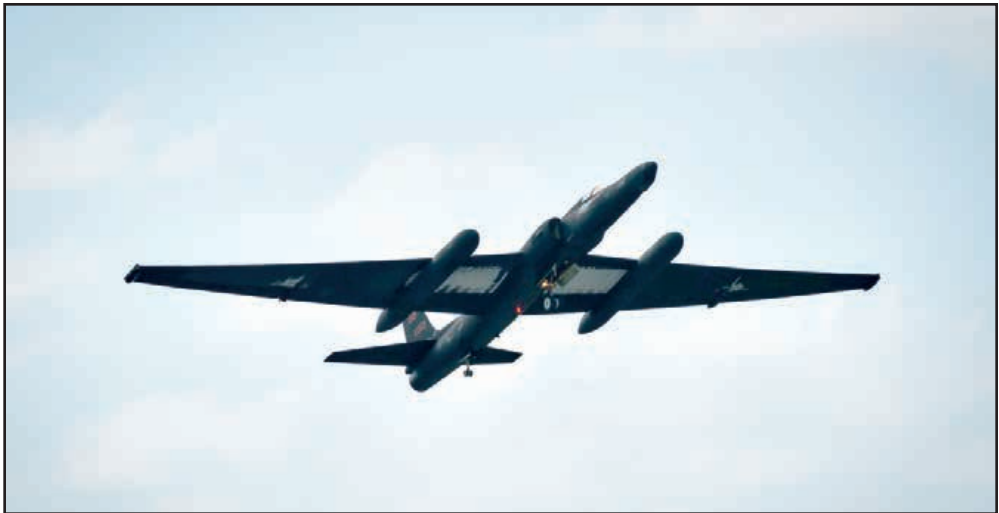
U.S. Air Force photo by Airman 1st Class Matthew Seefeldt A U-2 Dragon Lady flies over Kadena Air Base Jan 23, 2019. The U-2 is a single-jet engine aircraft capable of providing day and night, high altitude all-weather intelligence gathering.
