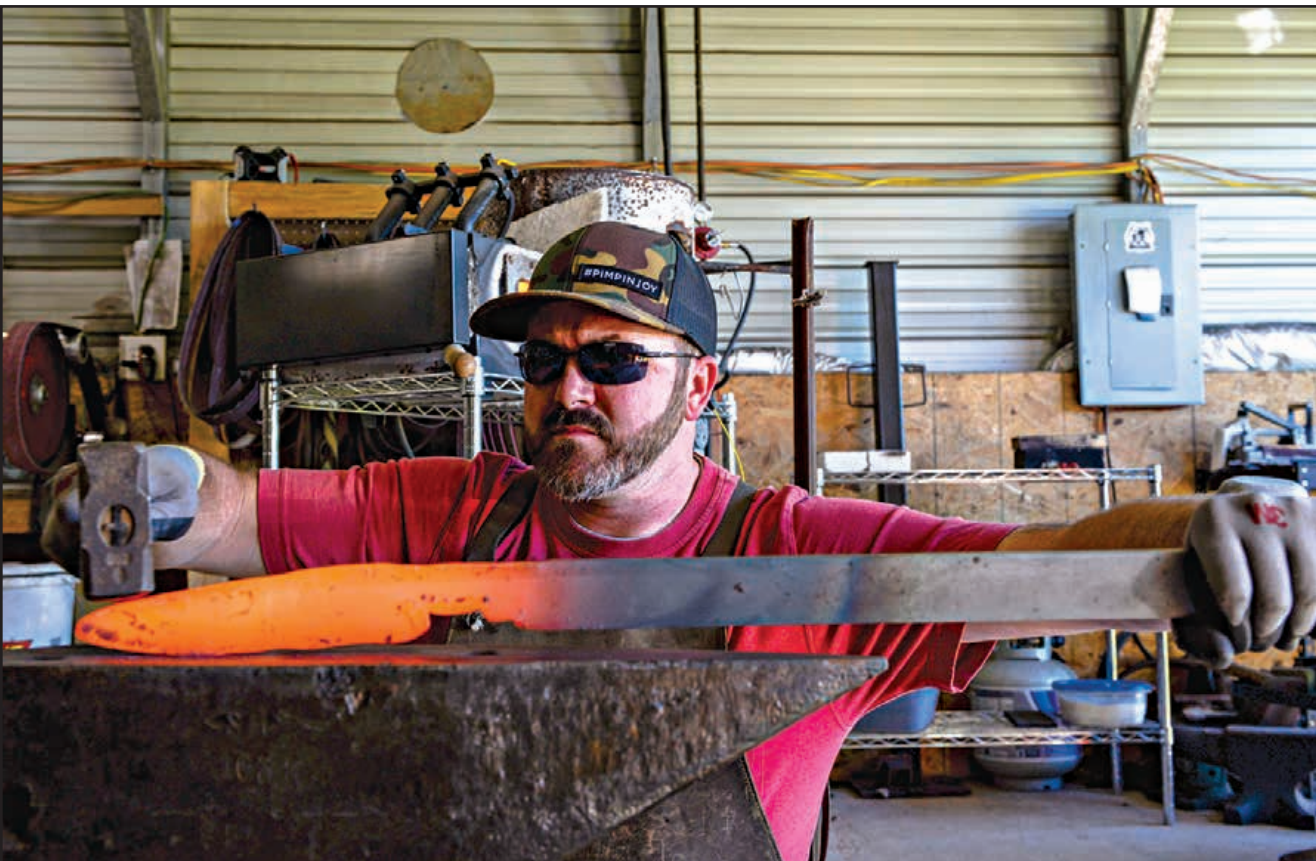
U.S. Air Force photo by Tech. Sgt. Christopher Gross Mitch Cargile gets eye level and hammers out the shape of a knife on his anvil April 15, 2020, at his home in Columbus, Miss. Cargile is a 14th Communications Squadron network technician at Columbus Air Force Base, Miss. Since 2013, he has taken up the art of knife making and forging.
