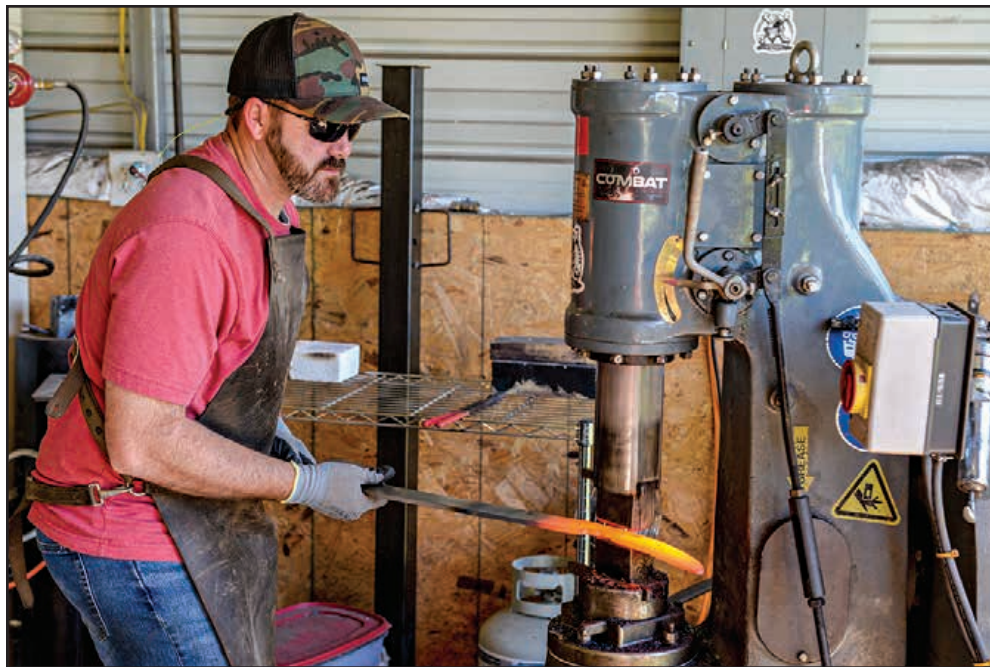
U.S. Air Force photo by Tech. Sgt. Christopher Gross Mitch Cargile flattens some steel on his power hammer as he creates the shape of his knife April 15, 2020, at his home in Columbus, Miss. Cargile is a 14th Communications Squadron network technician at Columbus Air Force Base, Miss. Cargile's blade making skills earned him a spot on the History Channel's "Forged in Fire," which aired Jan. 15, 2020.
