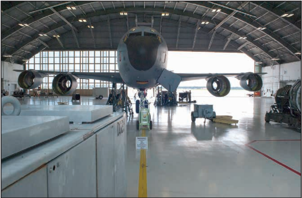
U.S. Air Force photo by Senior Airman Frank Rohrig A KC-135 Stratotanker aircraft rests on jacks during maintenance, July 3, 2019, at MacDill Air Force Base, Fla. A 6th Air Mobility Wing inspection team discovered a crack in one of the aircraft's trunnions and joined forces with Tinker Air Force Base's aircraft repair depot to fix it. This is the first time this type of maintenance has been performed at MacDill.
