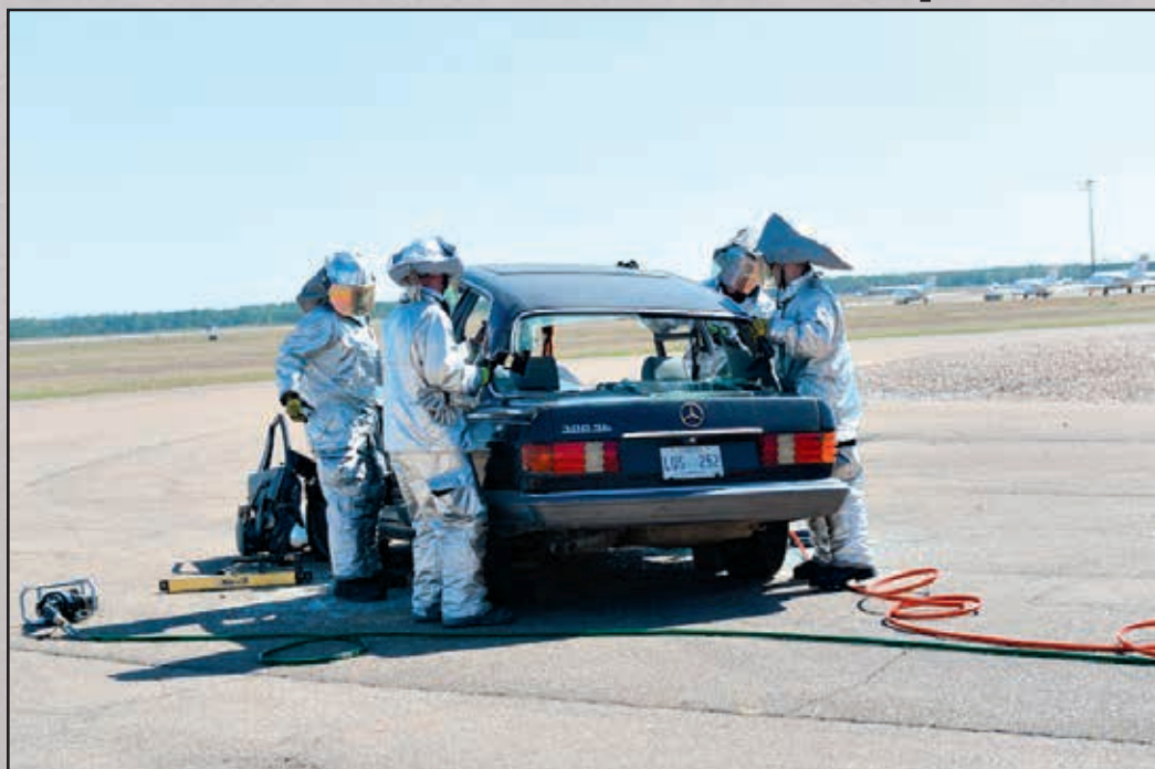
Firefighters use their tools to perform a vehicle extrication by removing the roof of a sedan Oct. 8 during the Fire Prevention Week open house at Columbus Air Force Base, Mississippi. Rather than remove the injured from the vehicle, firefighters are trained to remove the vehicle from the injured victim.
