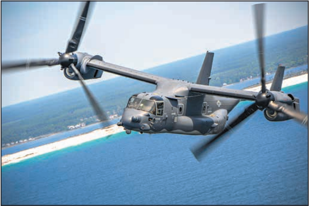
U.S. Air Force photo The CV-22 Osprey is a tiltrotor aircraft with the capability to perform both fixed-wing and rotary-wing missions. Its mission set includes long-range infiltration, exfiltration and resupply missions for special operations forces.
